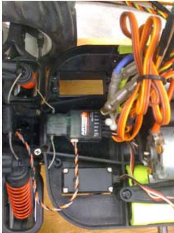
Figure 2: AR-7000 Receiver Installed
